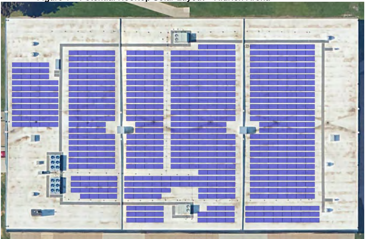
Figure 1 – Potential Rooftop Solar Layout – Aldrich Arena
