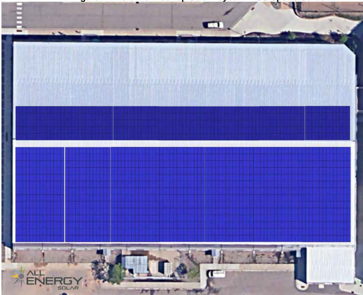
Figure 2 – Potential Rooftop Solar Layout – TCO Sports Garden
