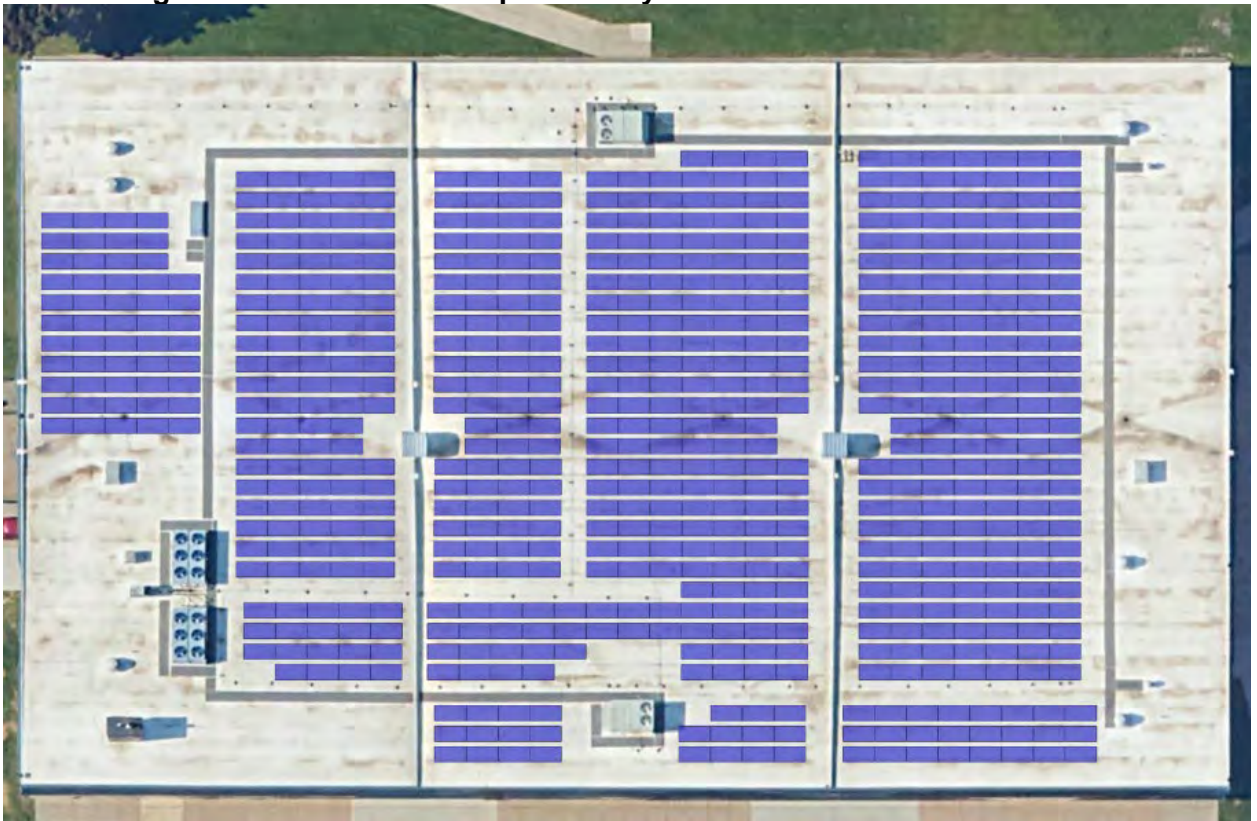
Figure 1 – Potential Rooftop Solar Layout – Aldrich Arena
